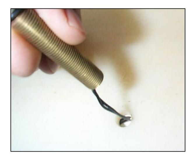
After inserting the sensor into the hole secure the sensor with the nut on the threaded portion of the sensor stud. Tighten the retaining nut until the O-ring seals between the boat and the sensor stud. The next photo shows the backside of the sensor with the nut installed.
