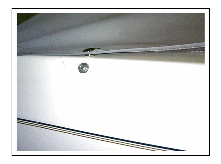
Repeat the above process until all the canvas snap sensor studs are installed. The next step is to place magnets in the canvas caps at the sensor locations. If a magnet is not in a cap when the cover is snapped to the sensor stud the alarm siren will sound one minute after the alarm has been activated. (One of the switches is open.)
