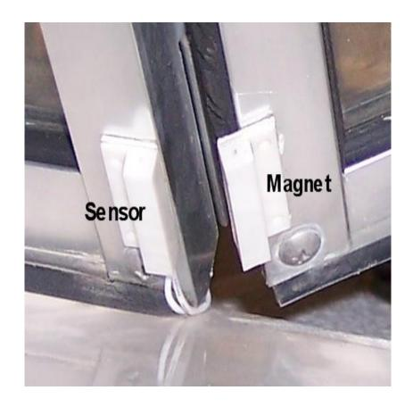
The magnet and sensor should be mounted so that they are not visible from outside the boat. These sensors are very effectively used on boat hatches and doors. The installation on a cabin door is similar to the window mounting as shown in the following photos.
