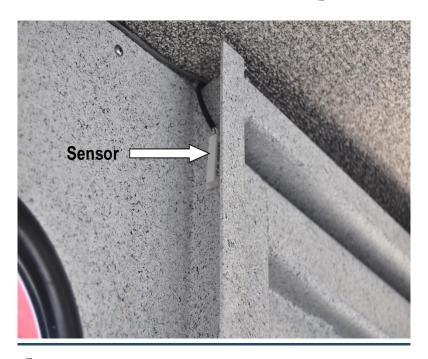
Hatch Sensor Magnet Location.
